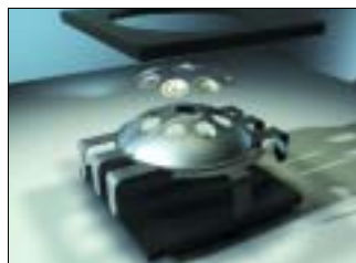
Fig. 3. After placing LED chips inside cups to create individual LED packages, these cups are positioned in a dome-shaped lead frame.
